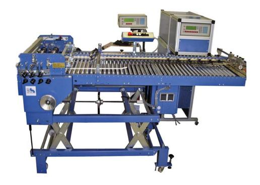
The 382 cutting unit from Herzog & Heymann is a very adaptable cutting machine. This machine can do many cutting functions, all that is needed is the appropriate knife. Because of its versatility there are a number of options available to the 382 that allow one to make the 382 cutting unit even more useful.
