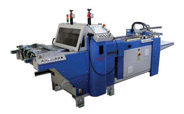
The BSR 550 Servo is able to process both single and folded products. Its innovative engineering allows it to process mailings, greeting cards, folded boxes, labels, and many other products in a one-up or multi-up production setting. Because of its flexible dies, the BSR 550 Servo can punch, cut, kiss cut, perforate, score, and deboss. This machine is a workhorse that can handle a wide variety of demands and produce excellent results every time.
